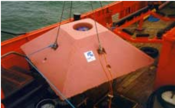
Fig. 2. ADCP installed in its mooring mount.
